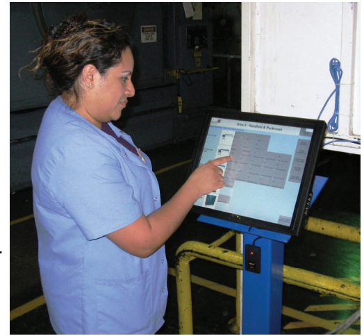
Using Spindle Direct Labor Module to login, associate to a piece of equipment and choose classification.
